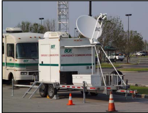
Portable Emergency Communications trailer as deployed in New Orleans, Louisiana following Hurricane Katrina in September, 2005. Data and voice resources were fed from the trailer to BGE's Mobile Operations Centre. [Ref 5]
