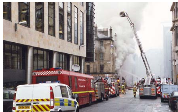
Forward command and control unit of Strathclyde Fire Service incorporating a satellite communications to link back to the Control Room and Corporate data network. (Picture courtesy of Excelebrate Technology)
